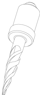
FIGURE 7: 1/16" CARVING BIT WITH PRESSED ON BUSHING
