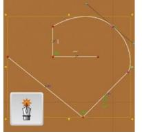
The Smart Spline tool is the most powerful drawing tool available to Project Designer. It allows you to quickly define a shape by placing points, or vertexes, along a path, while on-thefly designating the segments between as either lines or curves.
