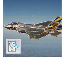
Import Tracing Image allows for an image file (jpg, png, gif, bmp) to be imported and placed on the design board to be used as a pattern for tracing with the drawing tools. The image can be cropped and scaled during the import process to suit your needs and can be toggled on and off to better view your drawing.
