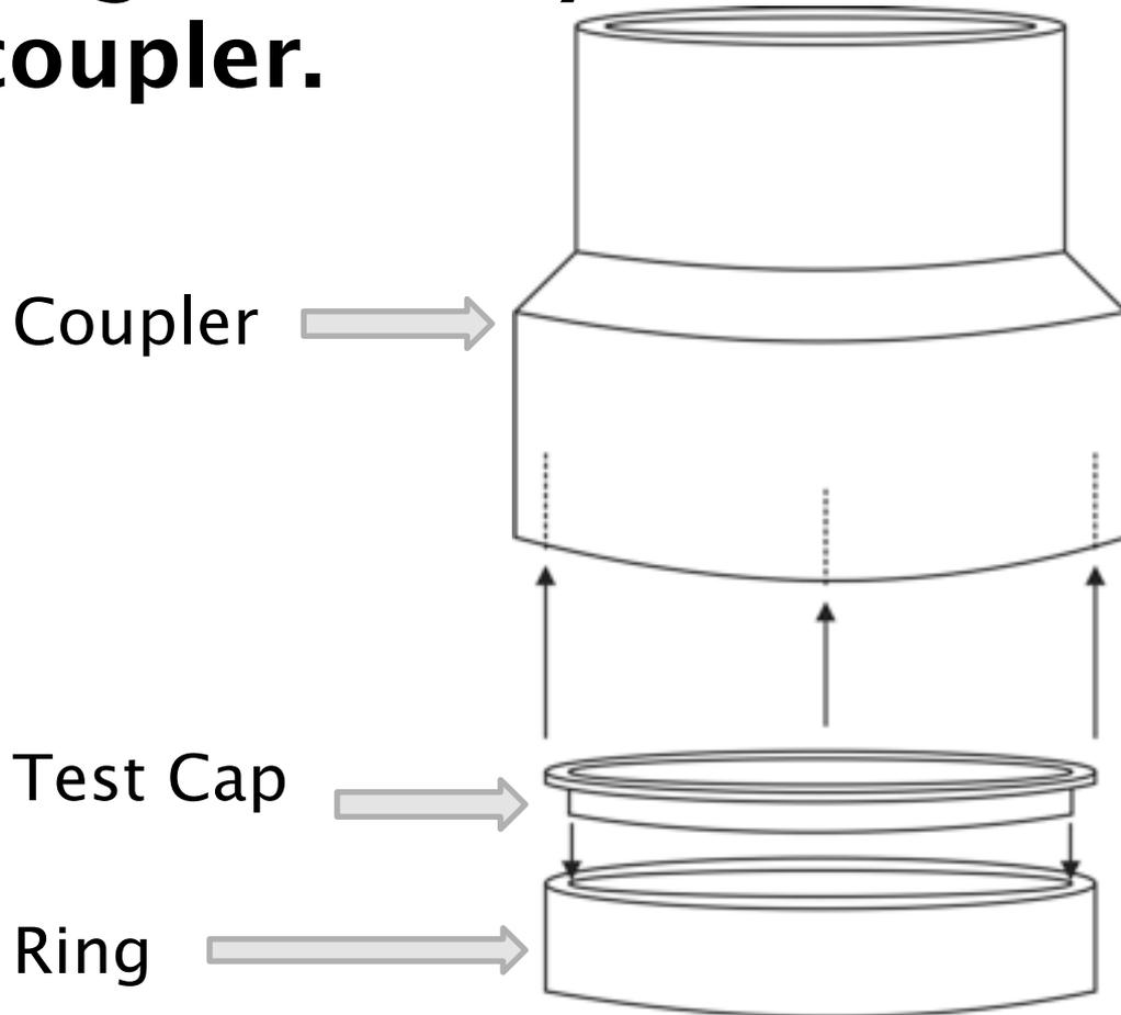
The fit should be snug. Secure from the inside with aluminum duct tape, if necessary.
