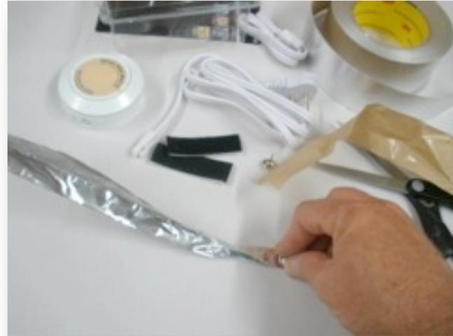
Plug in the A/C cord. Test by touching the metal tack. It should toggle the light to high, low, and off.
